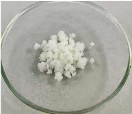
Figure 23. White polyhydroxyalkanoate (PHA) polymer recovered by solvent extraction from the rice paddy husk microbial consortium
