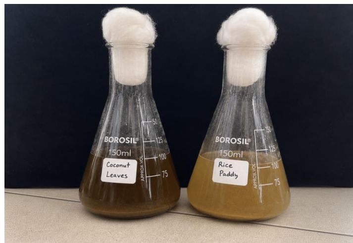
Figure 6. Preparation of submerged fermentation media using pre-treated coconut leaf or rice paddy as the primary carbon source.
