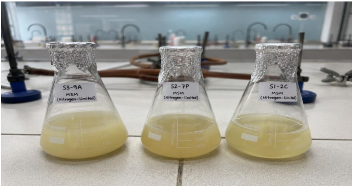
Figure 14. Submerged fermentation of the selected PHA-producing bacterial isolate in mineral salt medium under optimized culture conditions
