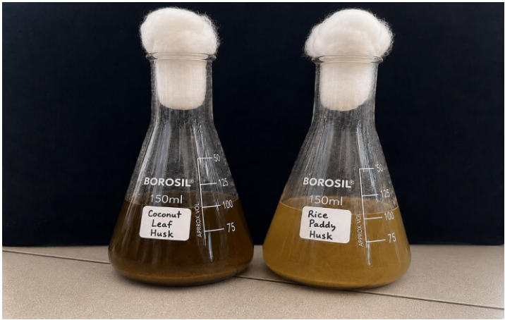
Figure 20. Development of the microbial consortium in agro-waste-based fermentation medium using coconut leaf husk and rice paddy husk as substrates under submerged fermentation conditions
