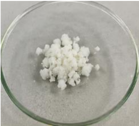
Figure 19. White polyhydroxyalkanoate (PHA) polymer recovered by solvent extraction from the selected Bacillus isolate
