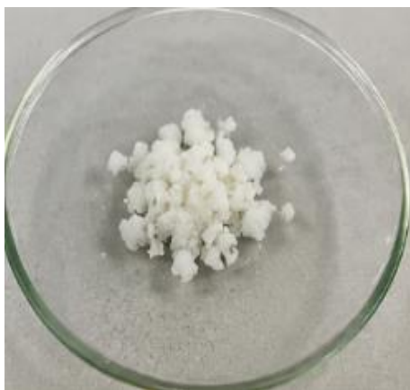
Figure 26. White polyhydroxyalkanoate (PHA) polymer recovered by solvent extraction from the coconut leaf husk microbial consortium
