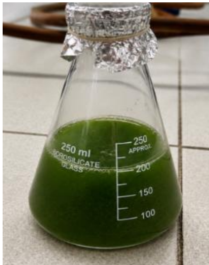
Figure 8. Microalgal culture cultivated under laboratory conditions using bicarbonate-supplemented growth medium
